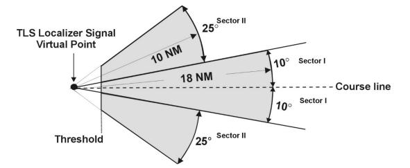
Localizer Coverage in Azimuth
