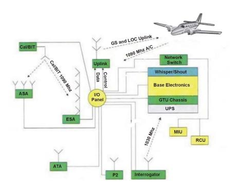
Figure 2-1 TLS Block Diagram
