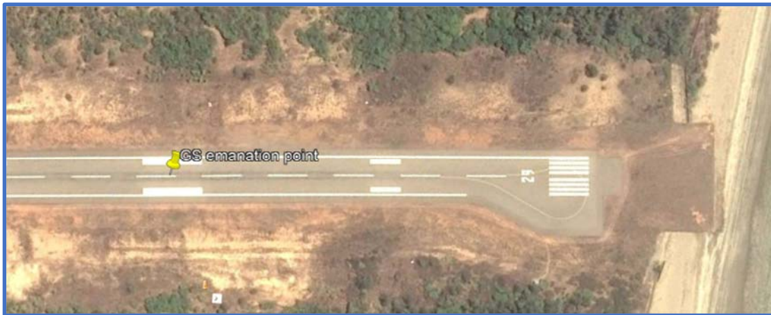
Figure 6 –TLS glide slope emanation point for a 55 TCH, 3.0 glide slope and 1049 foot distance from threshold
