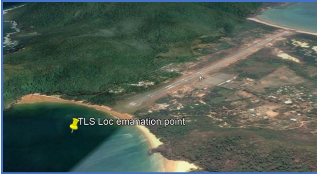
Figure 5 - Example of TLS localizer emanation point with an 8,016 foot distance from threshold
